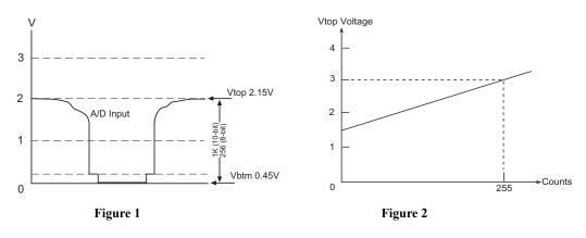
Vref2) is between 1V and 0.2V. The controllable range of the reference top voltage (Vtop) is between 1.5V and 3V.
